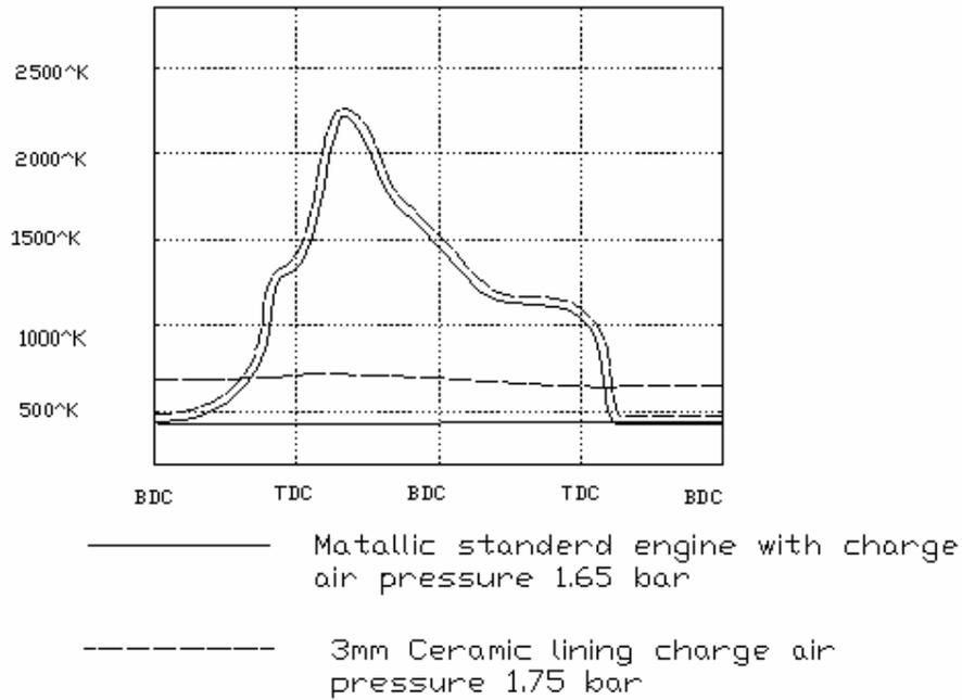
**Figure 3.a:** Typical gas and wall temperature profile of basic diesel engine and LHR-Engine [Randolph et. al., 4]
