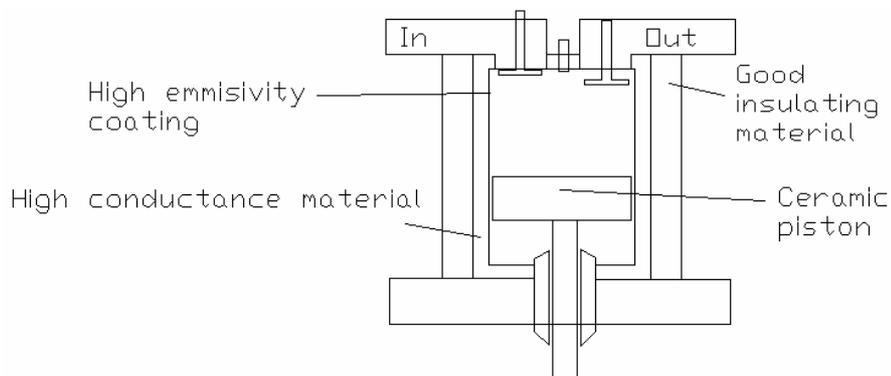
**Figure 2.a:** Typical construction schematic of LHR Engine [Randolph et. al., 4]
