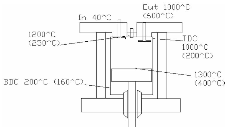
**Figure 2.b:** Typical temperature profile of basic diesel engine given in parenthesis and LHR engine temperature profile is shown without parenthesis [Randolph et. al., 4]
