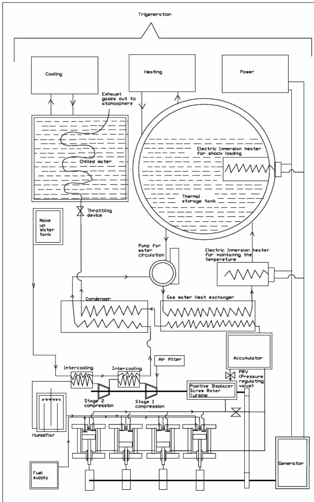
Figure 3.2a: Cycle network for LHR-engine based trigeneration system
